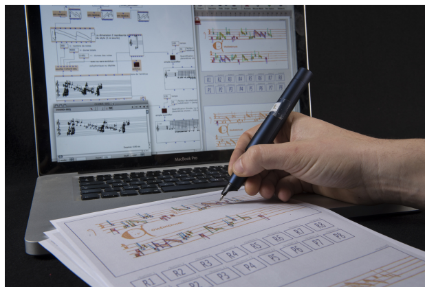
Figure 1: pOM in action. Pen events on the paper interface trigger musical processes in OpenMusic which and generate direct audio-visual feedback. Photo H. Raguet ©Inria.
