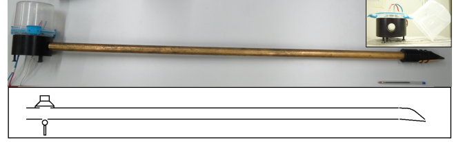
Figure 2: Top : Simplified bass clarinet (a cylindrical tube with a bass clarinet mouthpiece and a reed) with embedded control system with collocated microphone and speaker. Top right corner : control system removed from the instrument. Bottom : Schematic view of the instrument with embedded control system.
