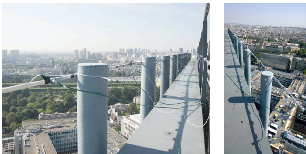
Figure 2 - Photographs of the linear antenna used for our study
